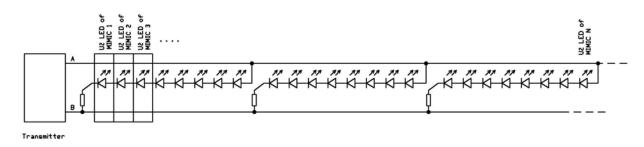
Fig. 8 . Each LED is actually an optocoupler of a MIMIC module.
