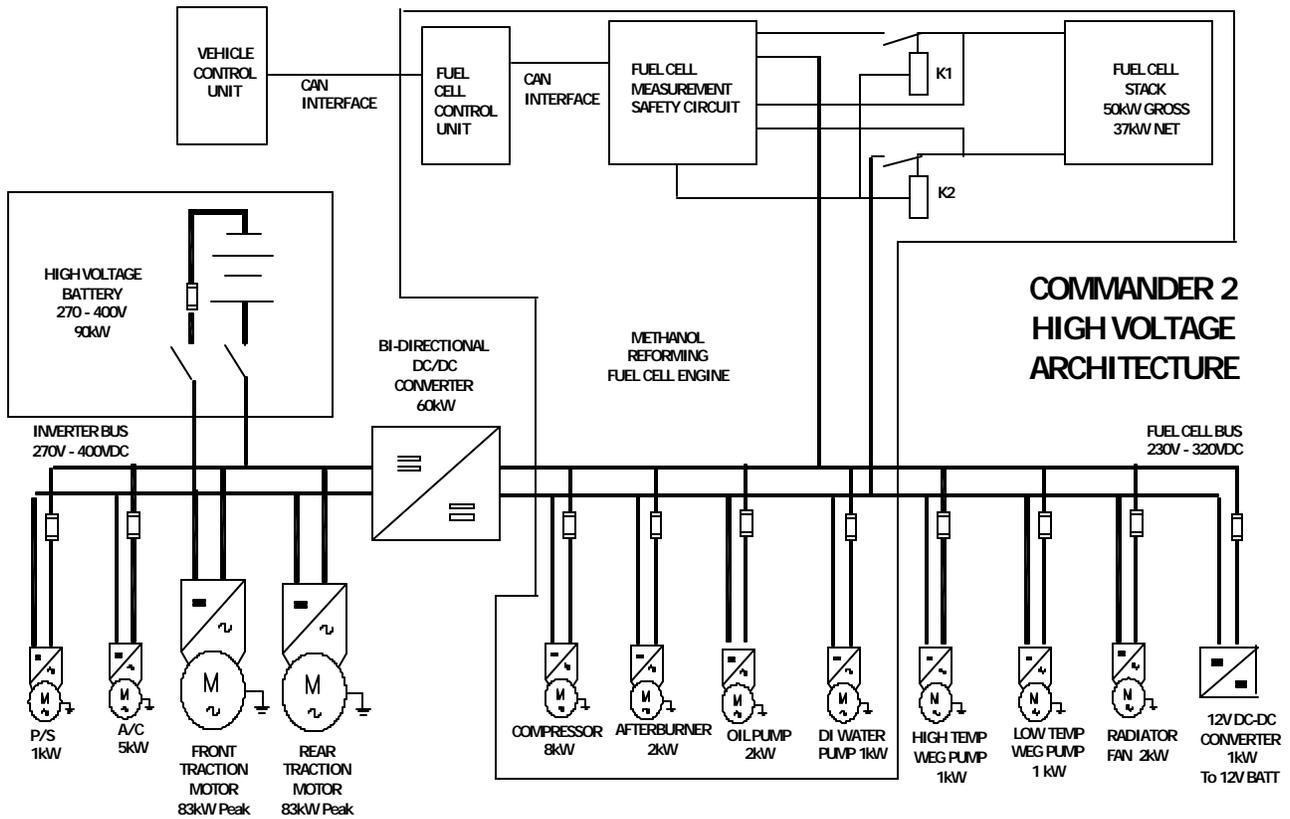
Figure 5. Jeep Commander 2 High Voltage Electrical Architecture
