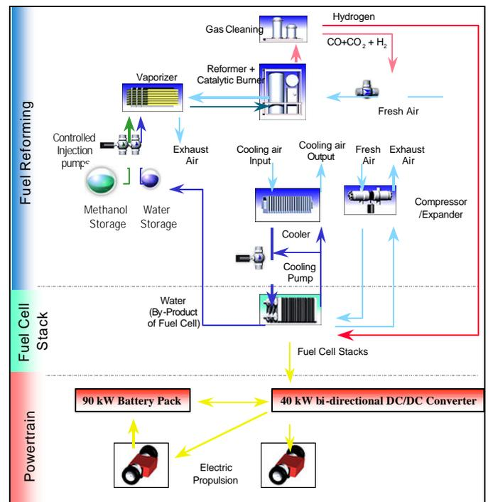
Figure 3. Jeep Commander 2 System Schematic
