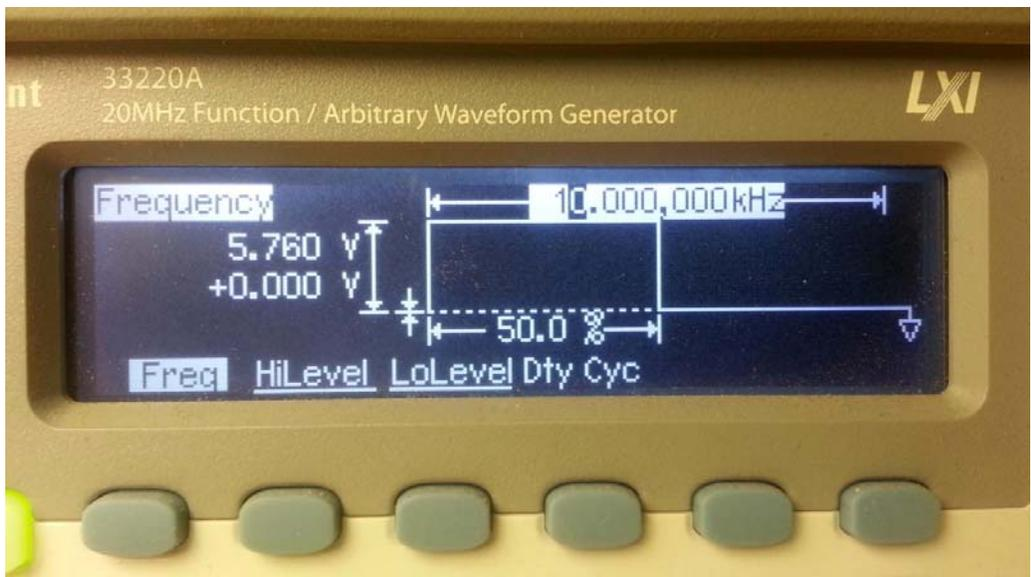
drop on the test leads. Because the scope was Kelvin connected to the test pads, I could dial required output to set actual voltage on the PCB to 5.000V. In my case it took 0.76V more to do that. Here is what the generated output looked like:
