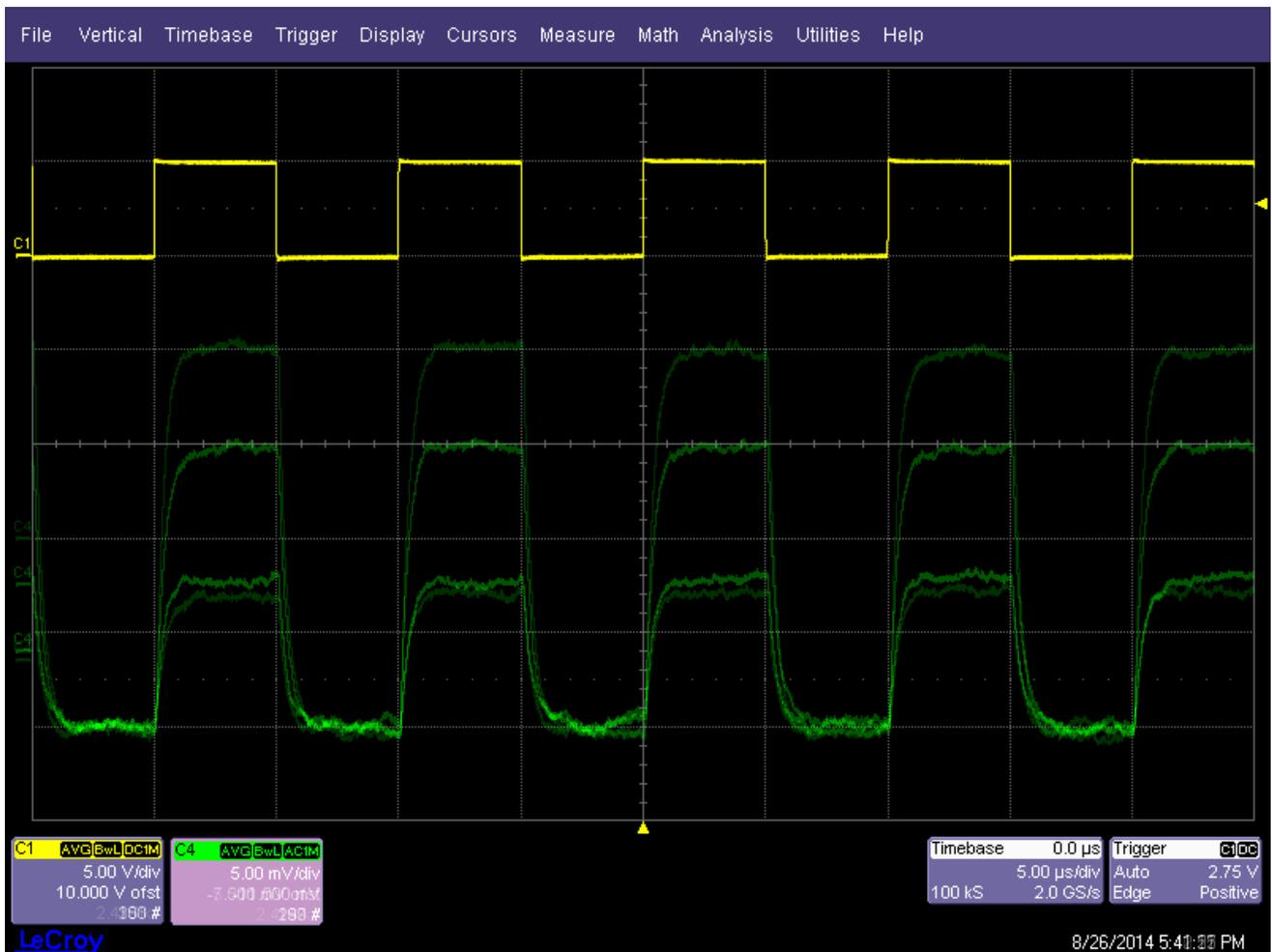
*20mA flowing through 0.5mm wide tracks located on different layers.*
