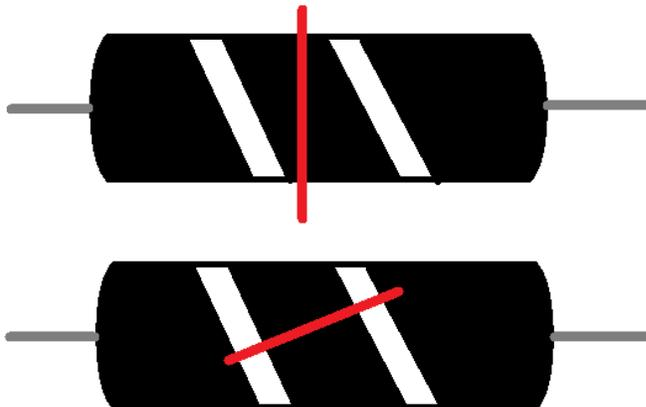
*This is what is happening. On the bottom sketch the tip is at proper 90° to the resistor's carbon track.*
