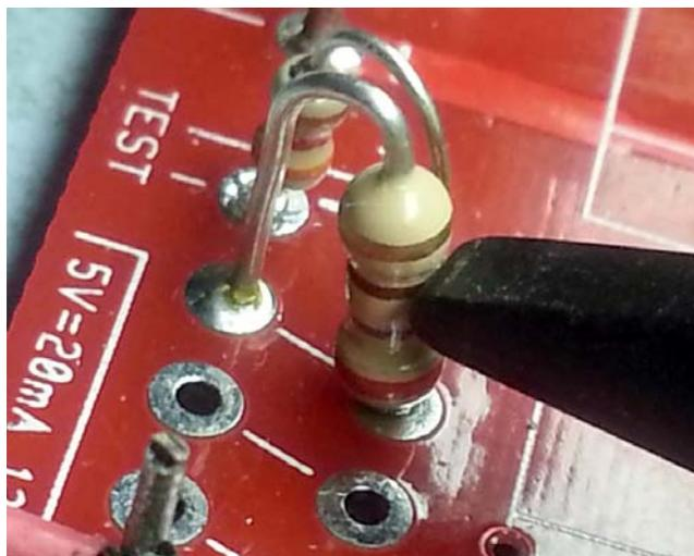
*Positioning probe tip for measurement.*
