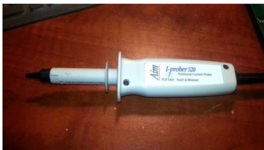
Fig. 10. Positional current probe
