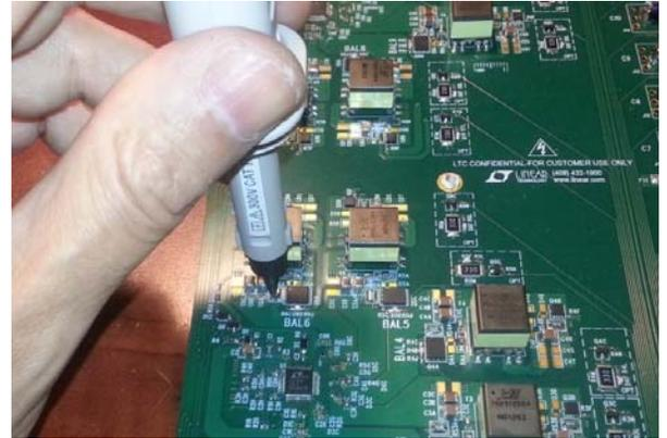
Fig.13. Using positional current probe
