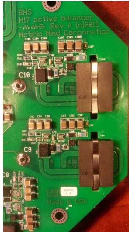
Fig.5. Planar transformer based design (fragment of Metric Mind corporation's M17 active balancer prototype PCB)
