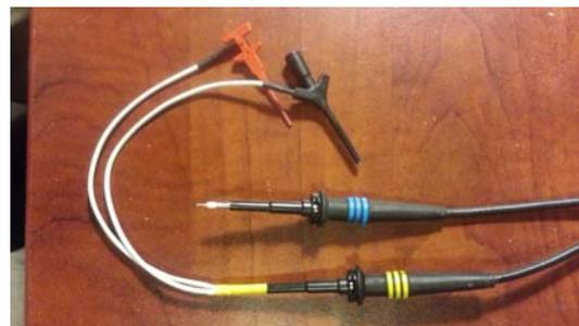
Fig. 6. This type of scope leads extension is absolutely unsuitable for high sensitivity probing.
