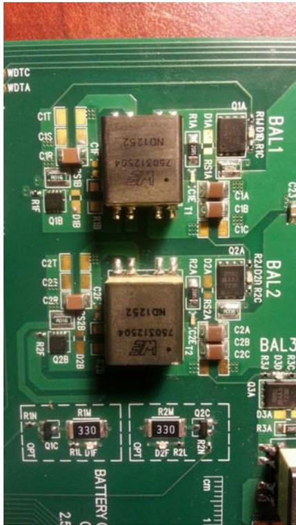
Fig.4. Wire wound transformer design (fragment of Linear Technology Corporation's 2100A active balancer demo circuit)
