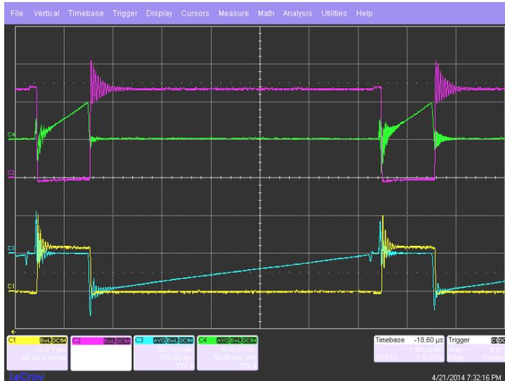
Fig. 8. Testing sense voltage (cyan trace) with direct connection of test leads to the current sense resistor.
